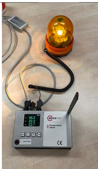
Beacon announcing the exceeding of the specified temperature
