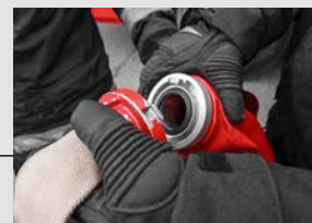
C52 Coupling (aluminium)
