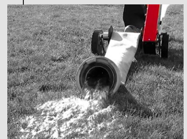
Use of the roller for draining residual water from the fire hose
