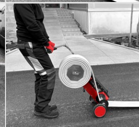
Roller 6 – walking winding – the weight of the hose is largely carried by the operator of the roller
