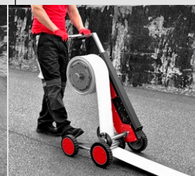
Roller 7 – walking winding – the entire weight of the hose is supported by the 4-wheel chassis
