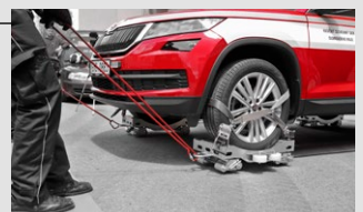
Manual transportation of a damaged electric vehicle with the help of transport trolleys
