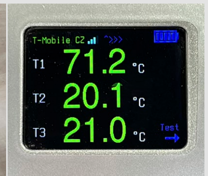
Temperature limit, overrun alarm – the device is sending a warning SMS
