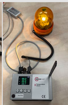
Beacon indicating that the set temperature has been exceeded
