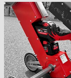
Roller is powered by 2 x 18 V Milwaukee batteries
