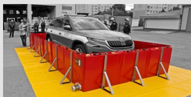
Container prepared for flooding of the car
