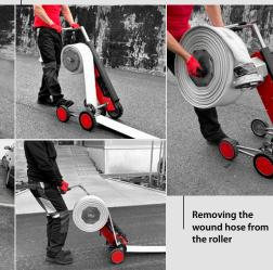
Roller 6 – walking winding – the weight of the hose is largely carried by the operator of the roller
