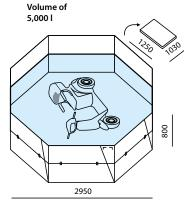
Extinguishing a damaged PV
