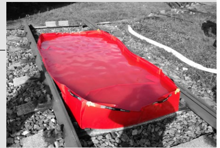
There are two ways to place the tank under a train or other track vehicle: across the tracks or along them into the inner space between the tracks. Both ways passed very strict testing.
