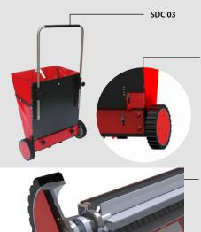
SDC 03 Plus has a magnetic sorbent spreader plate. The cover is operated with the toe of the shoe and when moving upwards, it stops on special stops adjustable according to the sorbent spreading density requirement.
